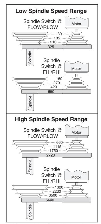
Figure 30. Model G0747 V-belt positions.
